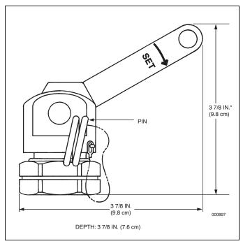
$<sup>^{\</sup>star}\,$  Add 1 9/16 in. (3.9 cm) to height when lever is in the straight up position.
